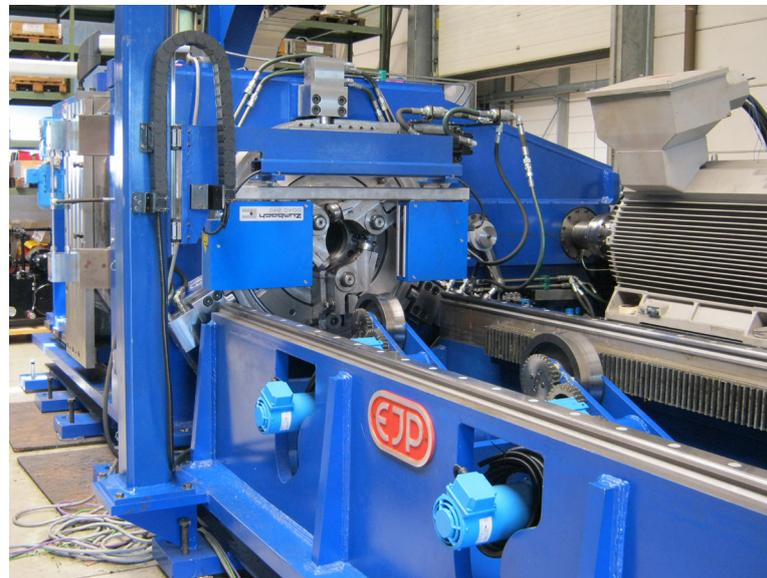
in the outer ring of the peeling head. The guide elements for the outer ring are eccentric, with the result that the spacing of the cutters from the centre axis is set precisely by a simple movement of the two components relative to each other.
